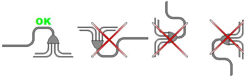
If a shaft is too long for the length required, it must be rolled up and never cut.
