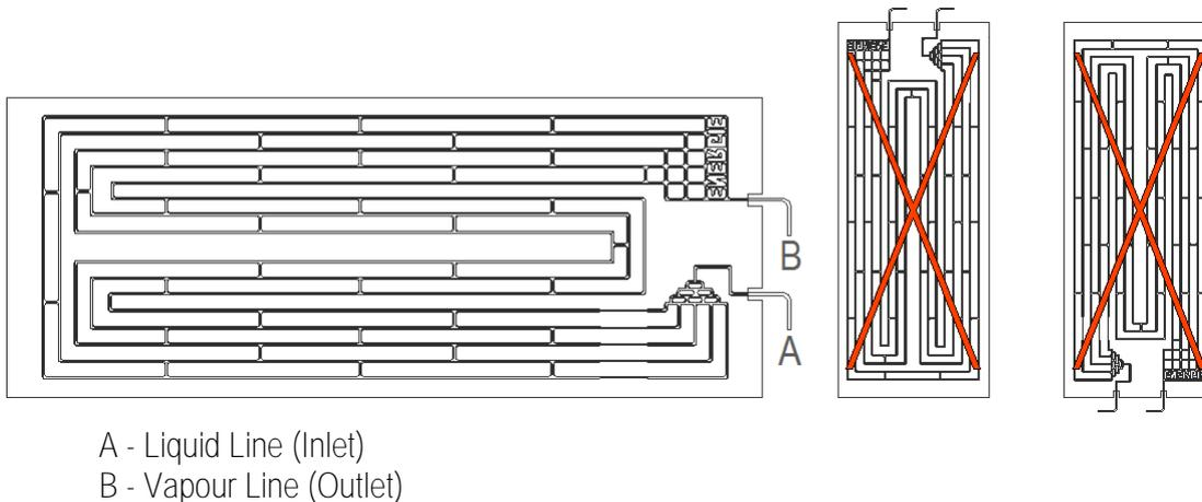
Right: A right-hand panel is installed on the left-hand side (front view). To this end, it has connections on right-hand side.
