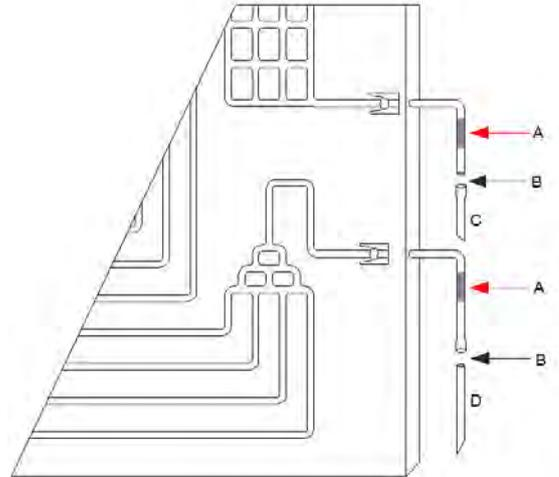
The copper is heated until it goes dark red at which point welding must begin. Bring the slightly inclined welding rod closer without exposing it to the flame. As a general rule, the quantity to be applied is the same as one and a half times the tube diameter. As soon as the alloy expands, stop heating and let it cool. As soon as the weld is in a solid state, you must cool the whole area around the weld immediately with a damp cloth.
