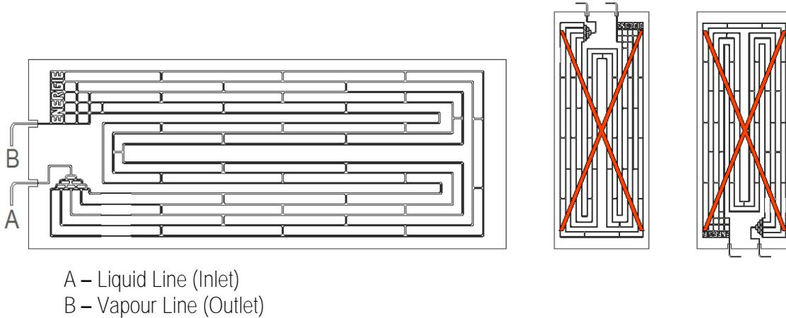
Left: A left-hand panel is installed on the right (front view). To this end, it has connections on the left side.
