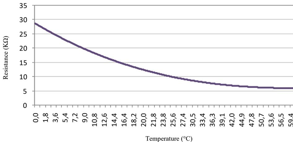
The installation of another temperature probe type will compromise the equipment operation, because the temperature values read by the controller will not be true.
