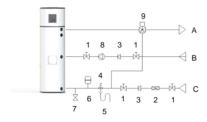
Heat source: water returning from heating radiators, district heating, etc.
