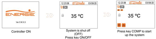
**Note 1:** The LED on the display indicates the status of your equipment. When is blinking means that your equipment don't have any order to work, if the LED is ON and no blinking, your system is working with the order that was given.
