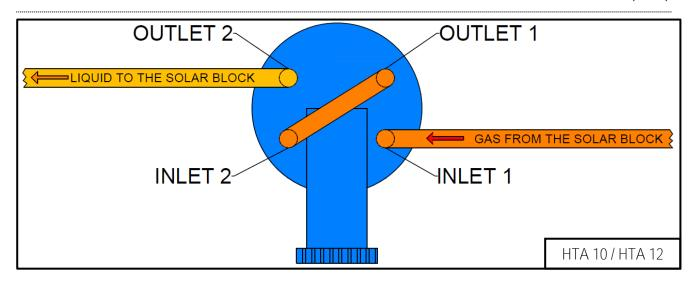
e) For the case of 2 heat exchangers, make the same type of connections (point d)) on each heat exchanger and make a derivation from the gas line that come from the solar block for the two Inlet 1 of each heat exchanger. Make the same type of connection for the liquid line of the solar block
