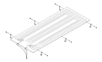
The affixation of the panels is ensured by aluminium supports\*. The support is bent in "L" form with two M8 through holes. The support base is secured to the roof (where applicable) using an M6 screw and a plastic plug or a female thread (depending on the situation).
