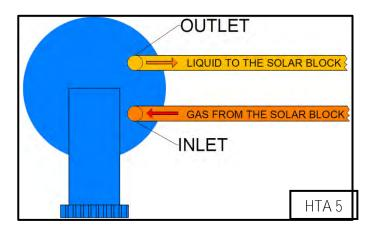
d) For the case of heat exchanger with 2 coils, weld the gas tube from the solar block to the Inlet 1 of the heat exchanger, weld a tube from the Outlet 1 to the Inlet 2, and finnally weld the liquid line of the solar block to the Outlet 2
