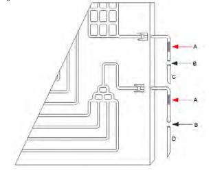
The copper is heated until it goes dark red at which point welding must begin. Bring the slightly inclined welding rod closer without exposing it to the flame. As a general rule, the quantity to be applied is the same as one and a half times the tube diameter. As soon as the alloy expands, stop heating and let it cool.
