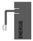
A 3/8" piping expansion area must be made, with the aid of an appropriate tool, for proper connection to the panel.
