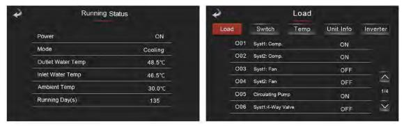
Figure 5- Heat Pump Operating Status
