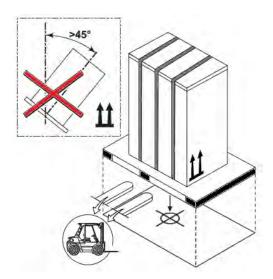
The recommended tool for transporting the unit while it is still on the pallet is a forklift. When transporting the unit, be sure to lift it only from the bottom and always with the unit placed on the pallet. Do not attempt to move the unit without assistance.
