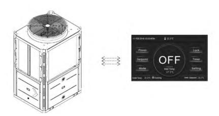
A cable comes with the equipment, which if it is not long enough and the distance between the outdoor unit and the display is less than 50 meters, we recommend installing a direct cable. The cable must have at least 4 conductors with a section of 0.5mm and protected with a shield to avoid interference, with a maximum length of 200m.
