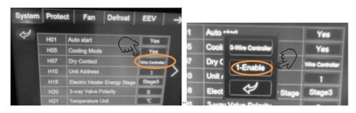
To change the configuration, click on the text "Wire controller" and a second window will automatically appear.
