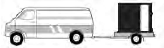
The BC must be transported to the installation location on a pallet. During transport, keep the equipment as level as possible, without tilting more than 45°.
