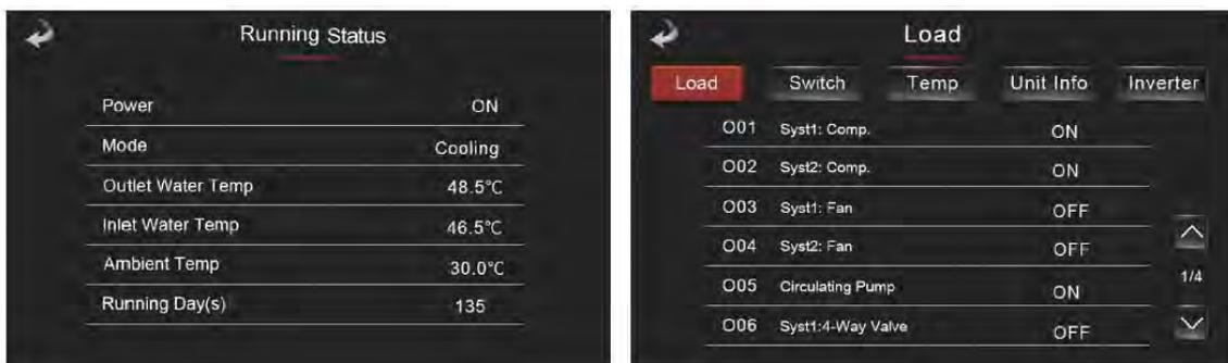
Figure 5- Heat Pump Operating Status
