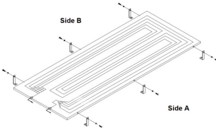
The profile shall be fixed to a base (e.g. a roof) via the provided plastic wall plugs and the self-tapping M6 screws. The M6 screws and the respective nuts and washers shall make the panel fixing to the profiles.
