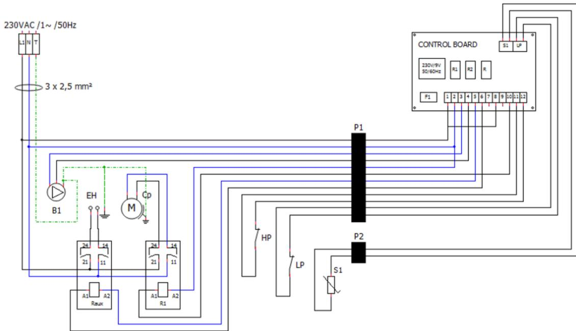
**NOTE: “EH” is not included on the equipment. It’s the responsibility of the installer to make its installation.**
