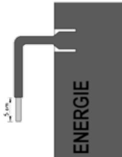
A 3/8" piping expansion area must be made, with the aid of an appropriate tool, for proper connection to the panel.
