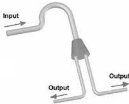
This distributor is placed between the two panels. The panel connecting pipes (1/4") must be exactly the same length, their extremities connecting directly to the panels.
