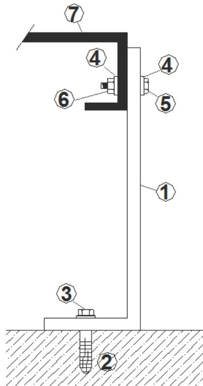
The system has 3 small profiles (side A) and 3 large profiles (side B) that must be fixed as shown in the image, giving the panel a desirable inclination.
